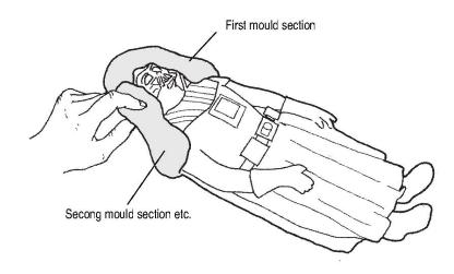
A release agent such as wax or silicon grease should be applied to the edges of each mould section before applying more Polymorph.
