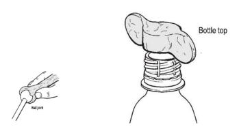
A threaded cap can be made by moulding Polymorph around a bottle top.
