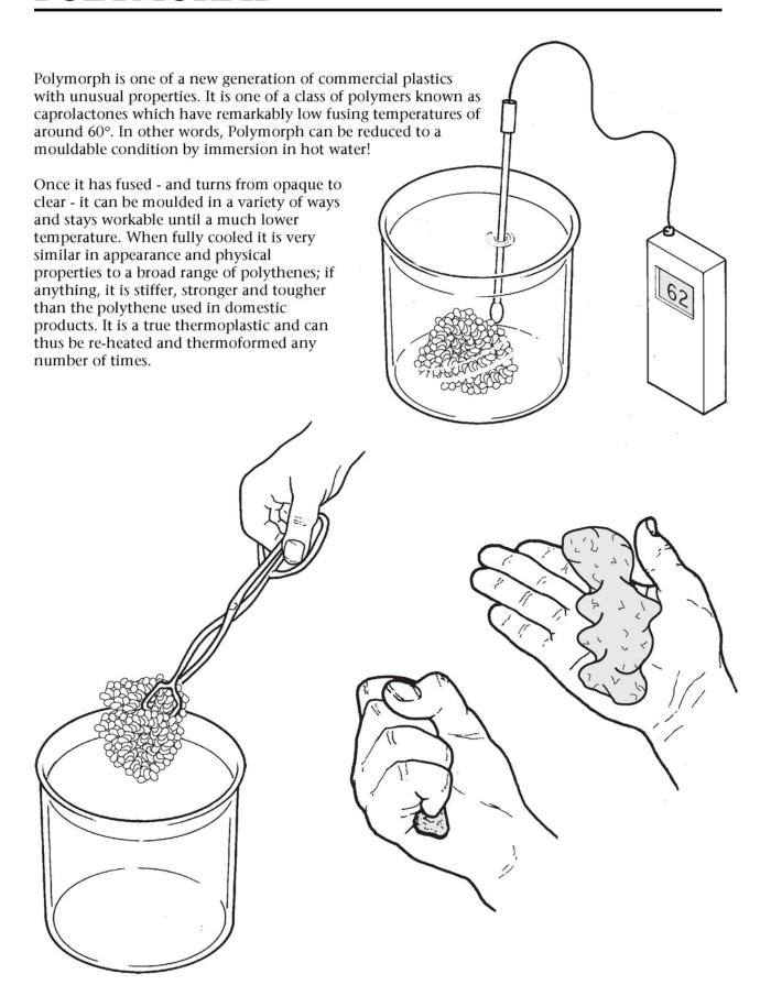
Polymorph is one of a new generation of commercial plastics with unusual properties. It is one of a class of polymers which have remarkably low fusing temperatures of around 60°. In other words, Polymorph can be reduced to a mouldable condition by immersion in hot water!
