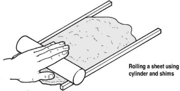
A uniform cylinder is created by rolling a mass of Polymorph between a flat surface and flat plate - both, ideally, warmed up. Bearing balls or rollers of a known diameter placed between the plates will provide a known diameter.
