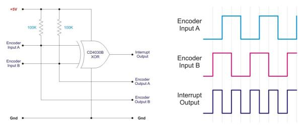
This allows a single interrupt pin to monitor both inputs of a quadrature encoder. Because the interrupt output is twice the frequency of either input it also allows speed and distance to be measured with twice the resolution.
